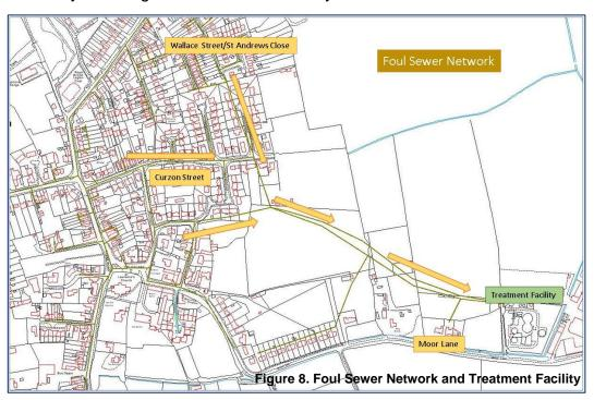
During the event on the 14th of November 5 properties were internally flooded by foul sewage water backing up and coming out of private drains. Early indications following investigations by Severn Trent Water suggest that there may be surface water ingress into the foul sewer system which is causing capacity issues.
