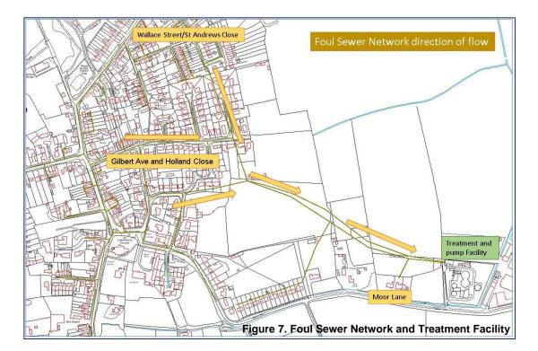
During the early hours of the 16<sup>th</sup>, foul sewage water backed up and spilled out of private drains and public sewer manholes in the highway. Severn Trent Water investigations have confirmed that there is some surface water ingress into the foul sewer system which is causing capacity issues.
