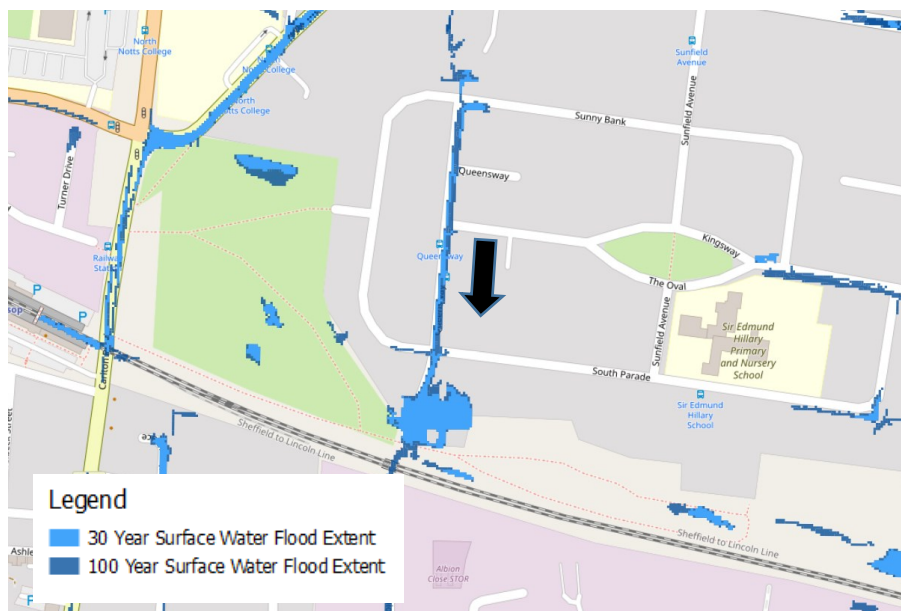
Figure 9. Predicted Surface Water Flood Extents – Queensway.
